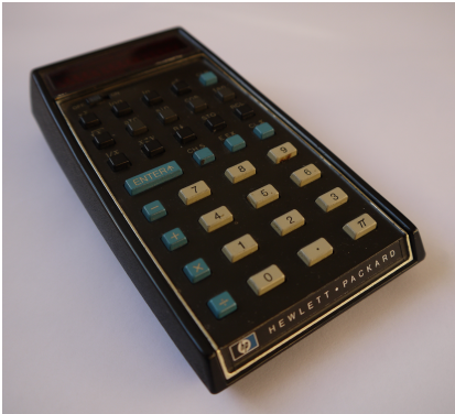
(a) The calculator outer casing, keypad and LED display.
